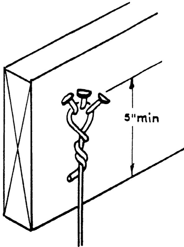
FIG. 2 Hanger Attached to Support Using Nails
