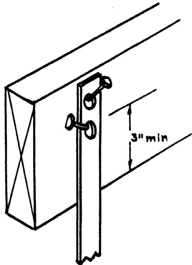
FIG. 4 Flat Hanger Attached to Support Using Nails
