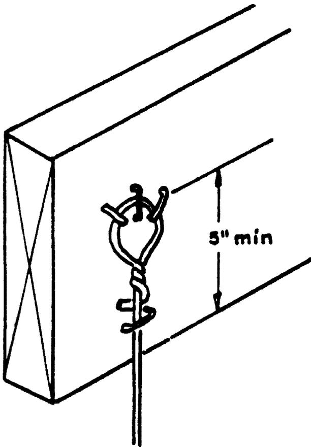
FIG. 3 Hanger Attached to Support Using Staples
